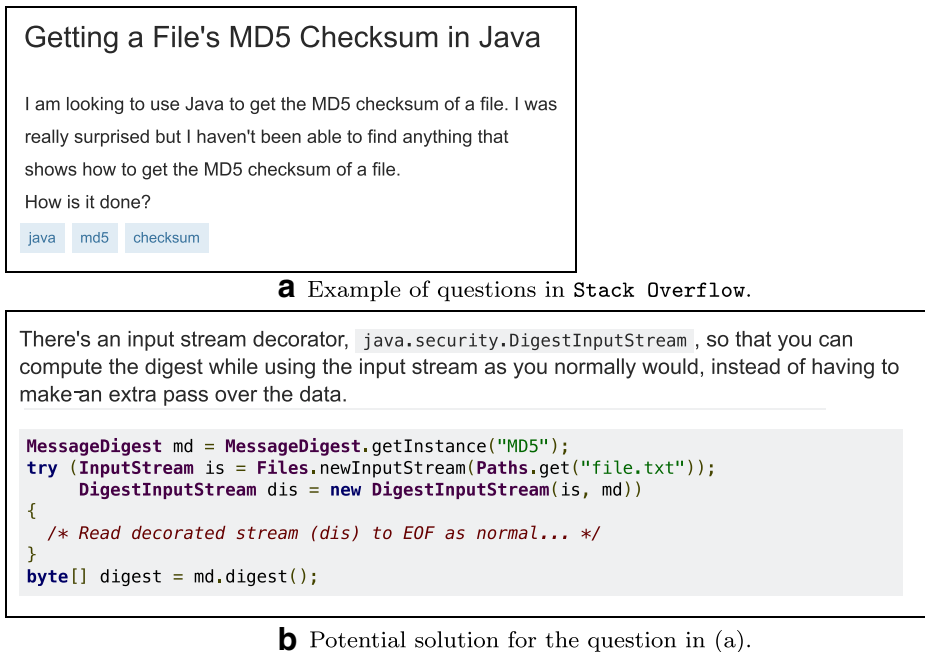
Fig. 1 Example of the vocabulary mismatch problem. Regarding the question shown in (a), a user of Stack Overflow posted a potential answer as shown in (b). The keywords of the question include MD5, checksum, Java, file. However, the snippet in the answer contains a different set of keywords such as MessageDigest, InputStream, DigestInputStream, digest, MD5, file. Using the keywords of the question when searching for code examples has significantly low possibility to locate code fragments similar to the snippet in the answer
